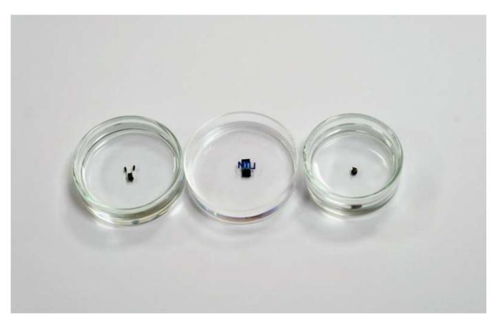
The NTU millimetre-sized robots measure about the size of a grain of rice and can be controlled using magnetic fields. Credit: Nanyang Technological University
